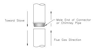
FIGURE 2.3 (A) Connecting Sections
